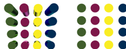
Left: non-telecentric optics Right: telecentric optics
