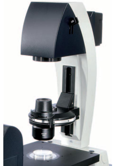
Transmitted light arm with integrated 30 W lamp house and compact S40/0.50 condenser, specifically for micromanipulation.
