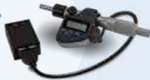
Digital micrometer* IMP-DIGMIC 25 mm travel
