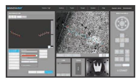
The distances of test points are automatically set to a minimum distance, following the standard, to assure correct testing is conducted. Time saving test mode "complete all indentations – then evaluate" and "auto-stop" to complete test series as soon as the lower hardness limit has been reached. Report Generator is enhanced with reporting features for this application.
