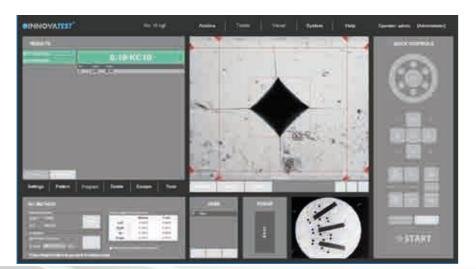
The software supports Kic crack detection under load with customized Kic result reporting. By way of one or both methods, Palmqvist or Median / Radial, fracture toughness is now a repeatable and reproducible test across multiple operators.
