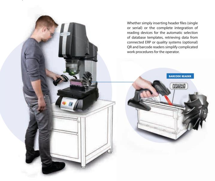
In the above application, a turbo part has been engraved with a QR code. Extra challenging was the fact that the QR code was engraved in a high polished part of the turbo shaft.
