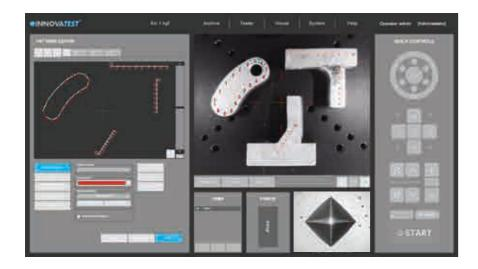
Combine different patterns and even different test forces in one program, and run them fully automatically. All test points can be identified individually or to customer specifications. The label is shown in the test result list and in the test results overview and in the results print out. An important function for sample analyses at the end of a test and in the future for review of previous tests.
