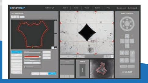
Subsequently, a limitless number of test points can be inserted into the scanned image, or be set at selected distances (offset), relative to the edge. This advanced feature enables the hardness testing procedure to be performed. An excellent featured combined with 2D or 3D hardness mapping, also known as "plane hardness chart".
