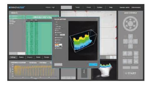
In addition to 2D graphic diagrams, the system can also automatically generate 3D diagrams. 2D and 3D hardness charts are included in one application.
