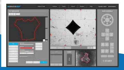
Subsequently, a limitless number of test points can be inserted into the scanned image, or be set at selected distances (offset), relative to the edge. This advanced feature enables the hardness testing procedure to be performed c. An excellent featured combined with 2D or 3D hardness mapping, also known as "plane hardness chart".
