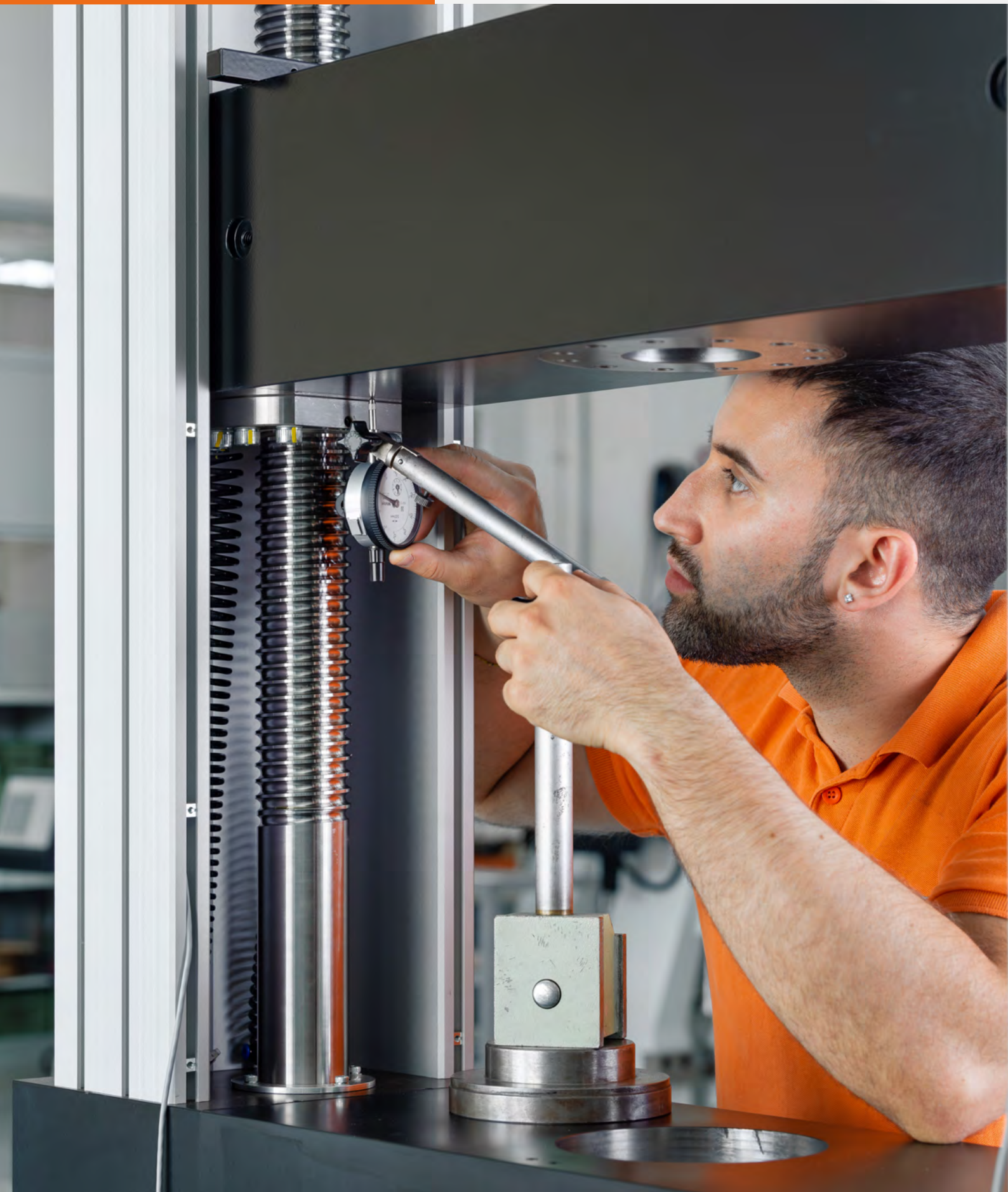
Ballscrew detail and crosshead alignment monitor
