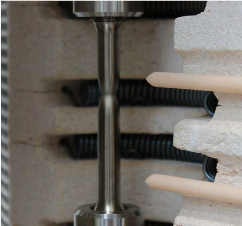
Hot temperature test with furnace according to ISO 6892-2
