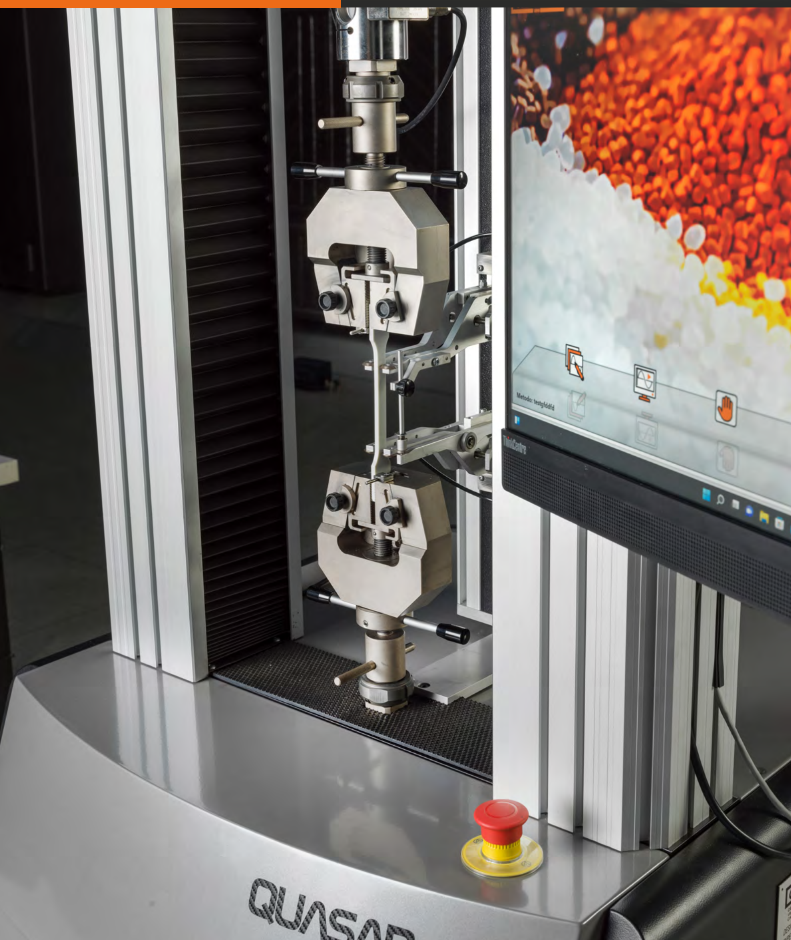
Tensile test on rigid plastic with MicronXT extensometer according to ISO 527-1 Standard
