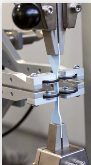
Extensometer knives suitable for plastic specimens
