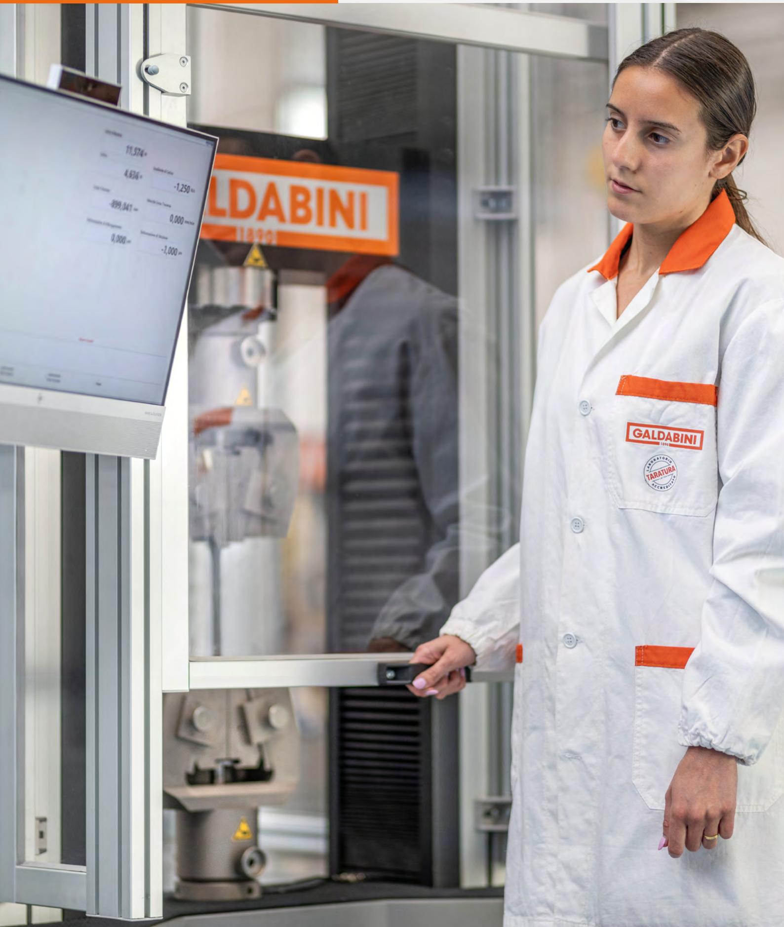
Safety barrier with sliding door
