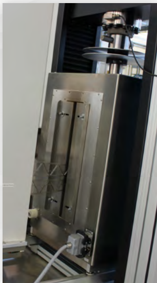
Micron Motor MFX extensometer input for hot tests with thermal chamber integration
