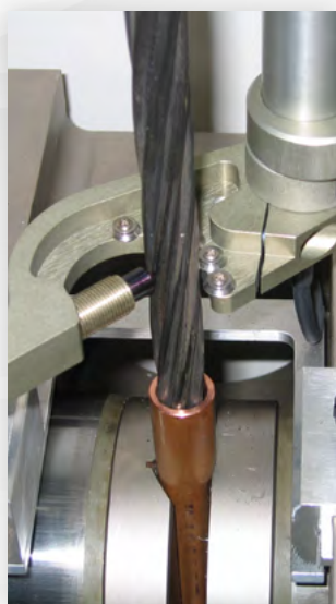
Extensometer for testing strands
