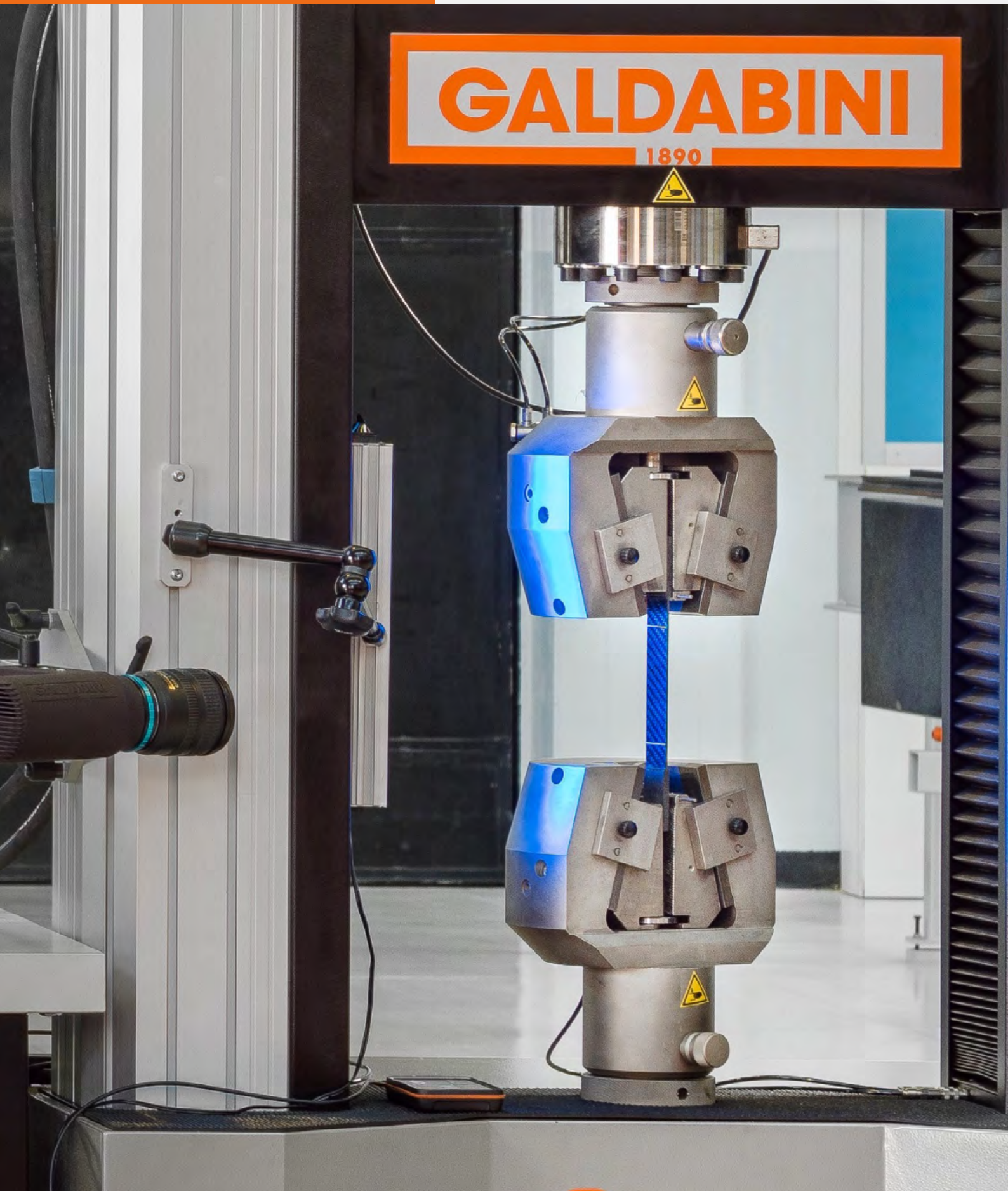
Tensile test with carbon specimen on Quasar 250 equipped with wedge grips and VideoXT
