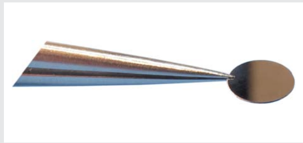
In such a manner, even hard and brittle materials can be thinned to be subsequently prepared for TEM investigation e.g. for ion thinning with the Leica EM RES101.
