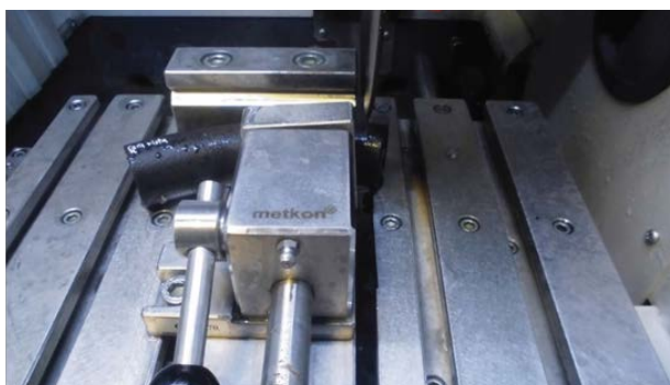
Number 1,2,4 samples are cut with DIMOS diamond blade.
