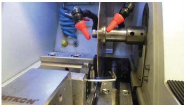
Number 1,2,4 samples are cut with DIMOS diamond blade.
