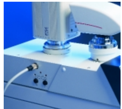
Motorized tube with two photo exits. The beamsplitter can direct the light either 100% to the eyepieces, 100% to photo exit 1 or 100% to photo exit 2.
