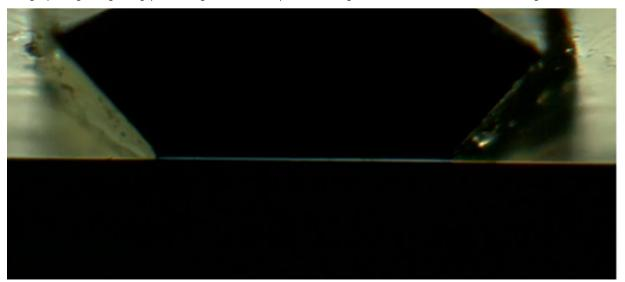
Using this method, an alignment with a deviation of less than 1 µm is possible over the entire block face. A blue light gap, where blue light is reflected from the block face typically indicates a distance of approximately 400 nm between the block face and the knife. An evenly distributed light gap across all angles at this distance is the most precise indicator of a correct light gap setting, which ensures minimal loss of material. The solution
