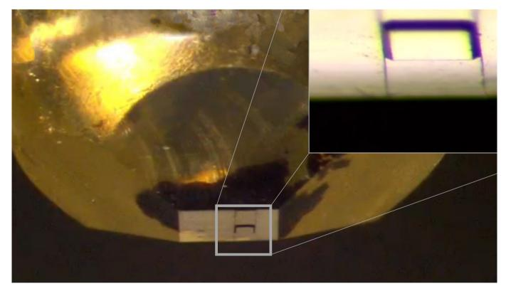
Figure 1: Final sample block after coarse and fine trimming. Magnified insert shows the final block face on top of the front face of the polymer bean. The front face was trimmed in a 45° shape using a milling device. The block face was trimmed using the microtome and a knife with 45° edges creating a pyramidal shape.
