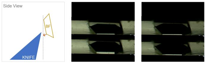
Figure 7: Adjusting the sample tilt. Left: Schematic drawing of the sample tilt principle. The sample is tilted until the block face surface is aligned to the knife edge along the cutting movement. Middle: Two images of the light gap when moving the sample up and down. The grey stripes do not have the same height. Right: The light gap after adjustment.
