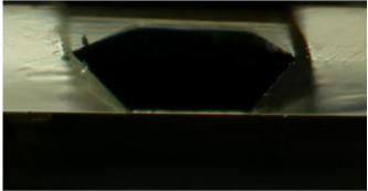
Figure 12: Final approach to the sample with safety distance of about 5 µm. Left: The user can decide to approach the sample automatically or manually after alignment. Right: Light gap after approach. A safety distance of about 5 µm will be kept.
