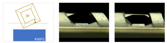
Figure 5: Adjusting the sample rotation. Left: Scheme of sample rotation versus knife edge. Middle: Sample not correctly rotated. Right: Sample correctly aligned to knife.
