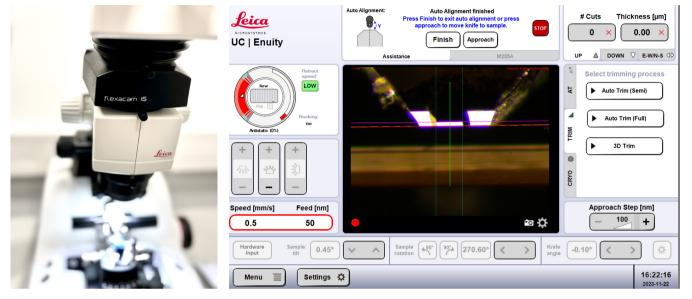
Figure 10: Built-in Flexacam i5 and screenshot of the touchscreen displaying the camera image with feedback lines for the automatic alignment (see below as well).
