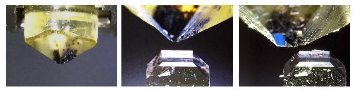
Figure 3: Fine trimming using a diamond trim knife. Left: Sample block after coarse trimming, before fine trimming. Center: The tip of the sample block before fine trimming. Below a 45 ° diamond trim knife is visible. Right: The front and the right side of the block face are already fine trimmed.
