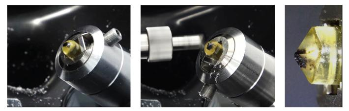
Figure 2: Sample block coarse trimming using the milling device EM RAPID. Left: Sample bean before trimming. Center: During milling of the second sector. Right: The final pretrimmed sample.
