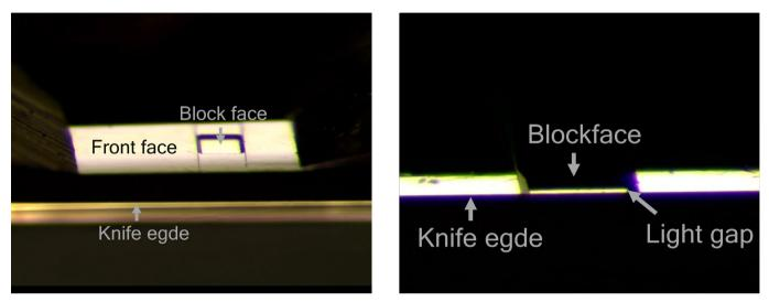
Figure 4: Reflection of the backside of the knife on the block face. Left: Overview, the light from below is reflected by the backside of the knife and is illuminating almost the complete front face including the target block face. Right: Approaching the block face with the knife, the reflection on the block face becomes a small stripe, called the light gap. The light gap serves as indicator for the orientation between knife and block face.
