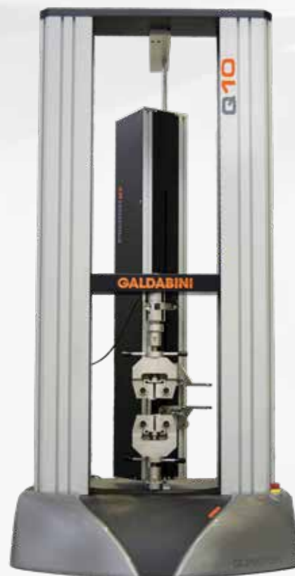
Universal testing machine Quantum 10 with Micron extensometer
