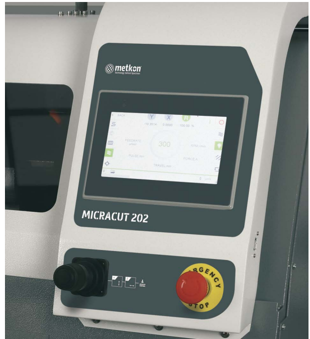
Coloured HMI touch screen controls with various cutting methods and database with cutting programs and maintenance monitoring
