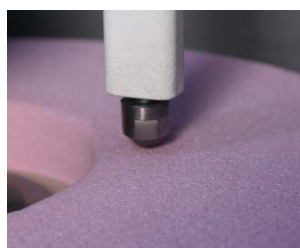
Automatic dressing of the grinding stone
